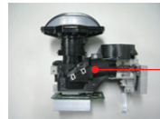
Key optical parts are shielded for dust protection.
